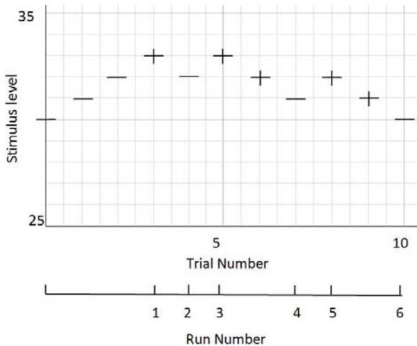
**Figure 6.** A sequence of stimulus level reversals during a 1-up 1-down staircase method. The initial value is typically determined based on preliminary experiments. The threshold of detection is calculated as the average of runs 2, 4 and 6 [16].
