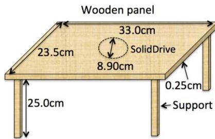
Figure 1. Schematic of the vibrating wooden surface.
