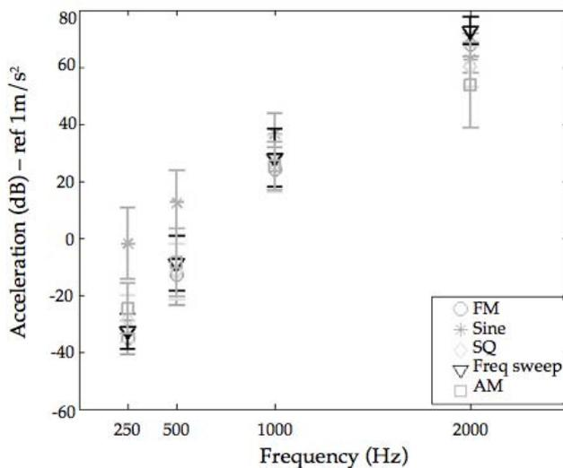
**Figure 7.** Threshold of vibration sensitivity to different signal types at different frequencies with 95% confidence intervals. (Note: The threshold for the AM tone at 2000 Hz was calculated with five data points because one subject could not detect that stimulus.)
