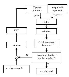
Figure 2. Frame-by-frame iterative phase estimation process
