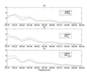
Figure 4. Magnitude spectra at a particular frame of a male speech vowel. Shown are comparisons between the original magnitude spectra and (a) RTISI at 5 iterations, (b) G&L at 5 iterations, and (c)G&L at 100 iterations.
