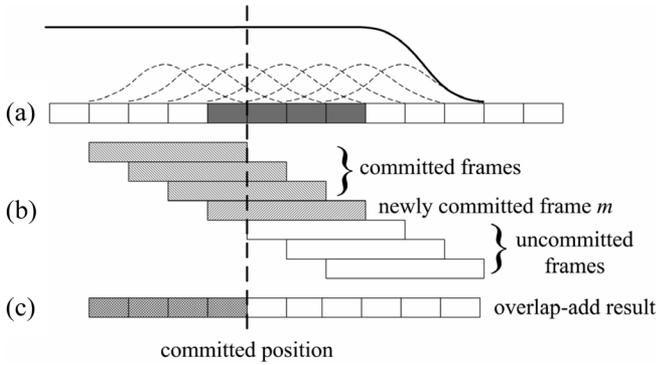
Fig. 3. RTISI with look-ahead after committing frame  $m$ . (a) The constructed signal with an indication of the contour (solid line) and overlapped windows (dashed line). (b) The frames currently in the frame buffer. There are three kinds of frames in the buffer: frames committed in the previous process; the newly committed frame  $m$ ; and the uncommitted frames. (c) The overlap-add result of the frames in the buffer. The shaded part is the fully committed signal ready for output.
