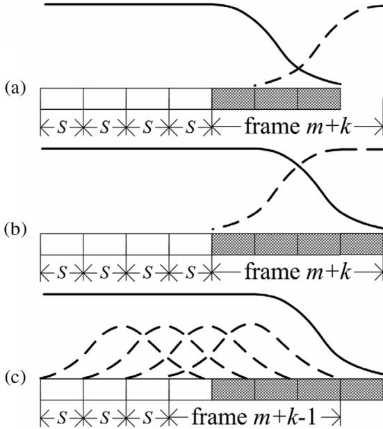
Fig. 4. Analysis windows, shown in dashed line. (a) The asymmetric window for the latest frame ( $m+k$ ) which is to be initialized. (b) Another asymmetric window for the latest frame ( $m+k$ ) which has been initialized. (c) The modified Hamming window for other uncommitted frames.
