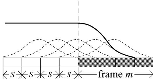
Fig. 1. Illustration of the partially reconstructed frames of signal  $y(n)$ . Before frame  $m$  is estimated, there exists an overlap-added result of the frames  $m - 1$ ,  $m - 2$ ,  $m - 3$  in the range of the frame  $m$  window. The solid line shows the time-domain contour of the previously constructed signal, and the dotted lines show the overlap-added windows. The shaded part is the range of frame  $m$ .  $S$  is the synthesis step size between two adjacent frames.
