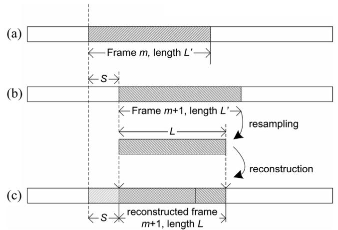
Fig. 7. Real-time pitch modification process. (a) Frame  $m$  in the original signal. (b) Frame  $m + 1$  in the original signal. (c) Frame  $m + 1$  in the reconstructed signal, which is obtained by resampling the original frame  $m + 1$  and synthesizing.
